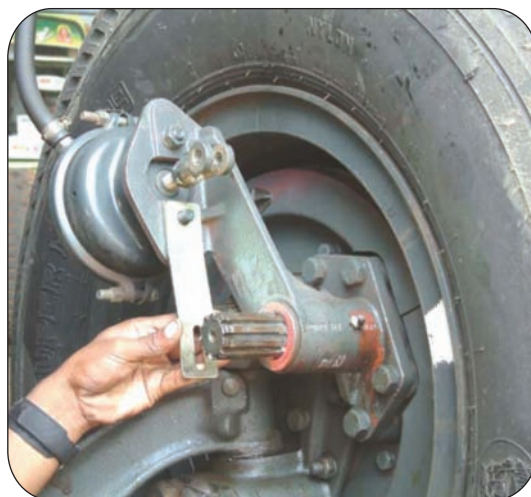
Initially fit anchor bracket loose at the brake chamber mounting bolt
