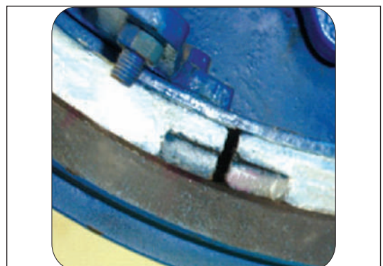
Close brake shoe clearance to drum to zero
