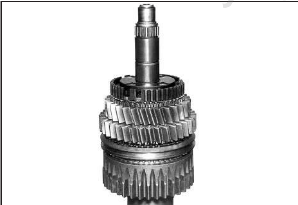
Heat synchro body and locate its slots on lugs of synchro ring.
