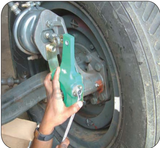
Align & fix clevis pin/bolt by rotating 12 mm adjusting hex
