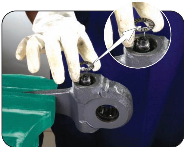
Assemble thrust bearing (4)
