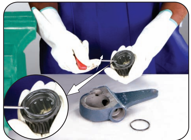
Remove sealing rings (15)
