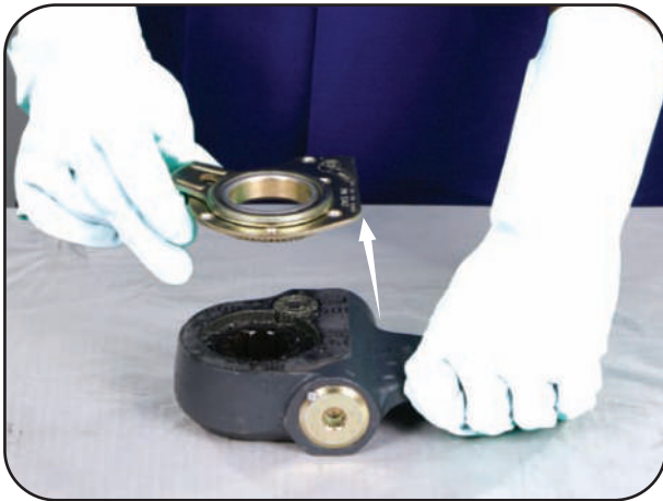
Remove cover plate assembly (17).
