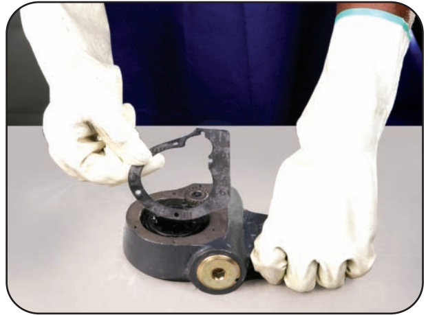
Assemble gasket (16) after applying grease on both faces.
