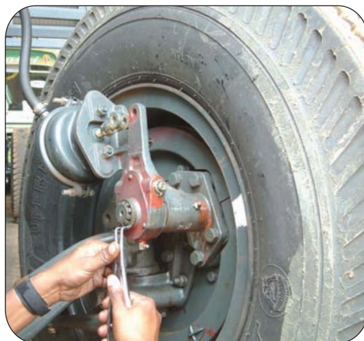
Remove circlip
