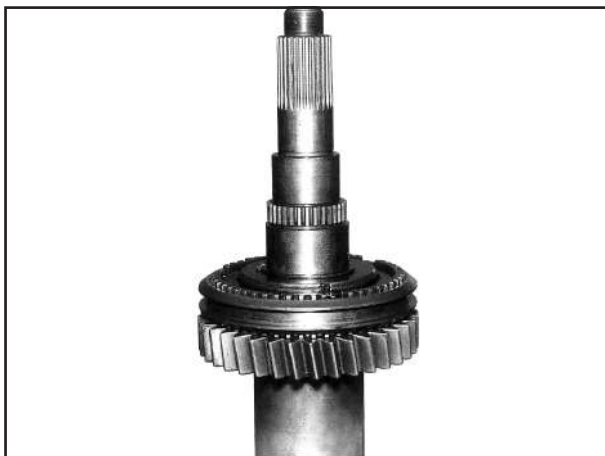
Fit sliding sleeve.
