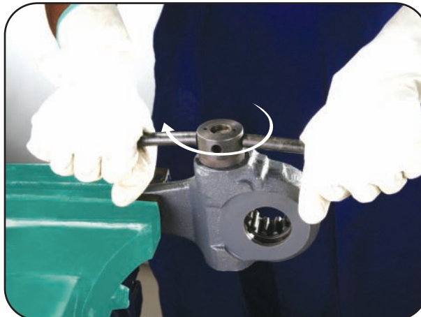
Tighten bearing retainer (2).
