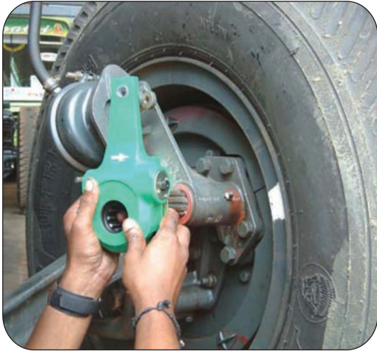
Fit SASA with arrow/adjusting hex away from the brake chamber
