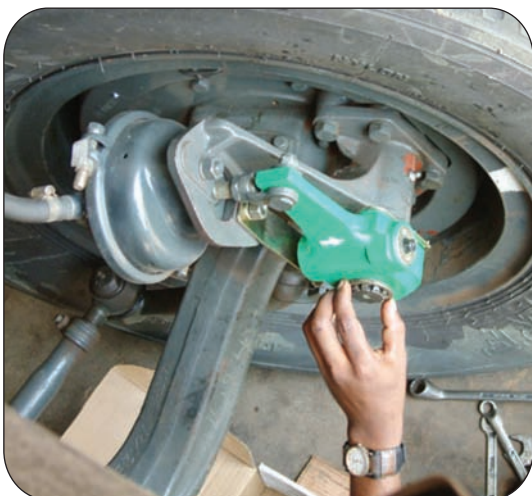
Fix circlip, ensuring 0.50 mm axial play on cam shaft.
