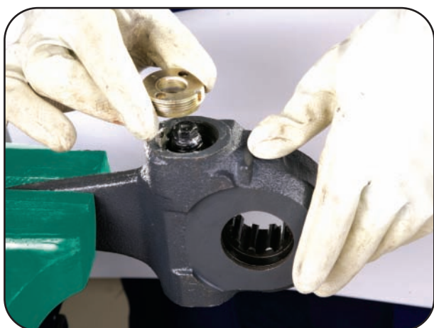
Assemble bearing retainer (2).
