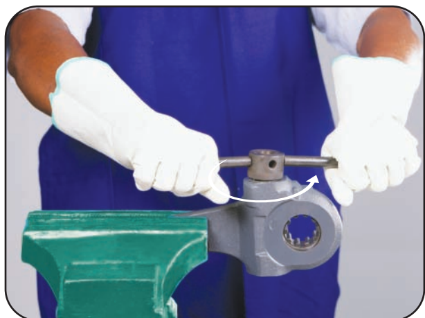
Remove bearing retainer (2)
