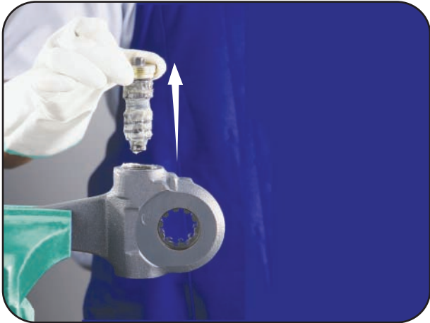
Remove worm shaft assembly
