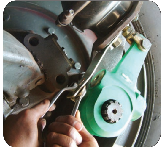
Align control arm bolt to anchor bracket and tighten
