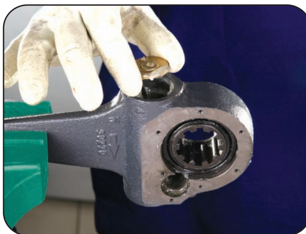
Assemble spring seat (9).
