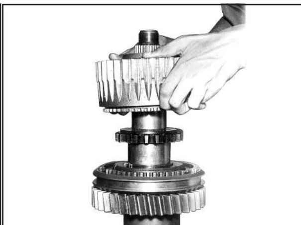
Heat (120°C) and fit spacer with rounded end of teeth upward.
