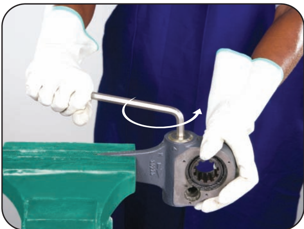
Remove spring retainer(11) with 10 mm allen key
