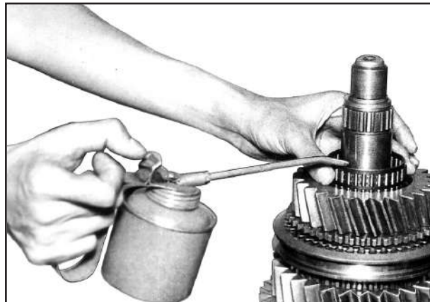
Lubricate needle bearing and fit.
