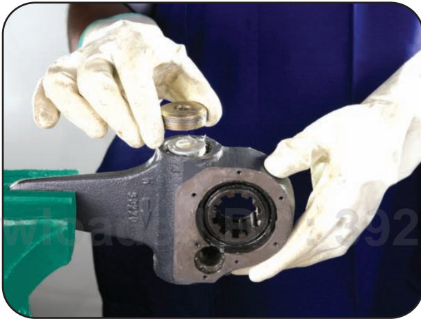
Assemble spring retainer (11) Tighten spring retainer (11) with 1 to 1.5 mm projection above the body face.
