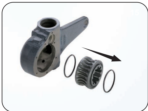
Body (8), sealing rings (15) and worm wheel (14)
