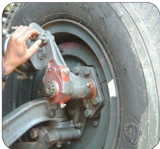
Remove clevis pin/bolt
