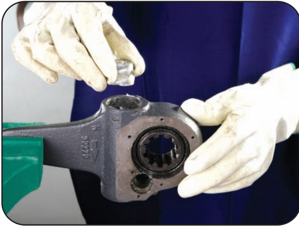
Assemble heavy coil spring (10)
