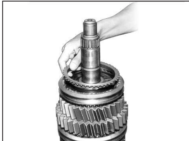
Fit 3rd synchro ring into slot of synchro body.
